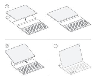
Note: The keyboard will only enter operating mode once the Pad and keyboard have been linked together correctly as shown above.
