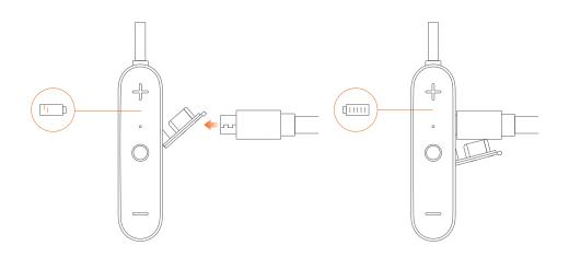
When the power is low, the light will turn red and start blinking. You'll hear a notification sound as well. Note: After fully charged, make sure the USB port is capped to prevent moisture.
