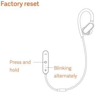
When the earphones are charging, press and hold the multifunction button until the light starts blinking alternately.
